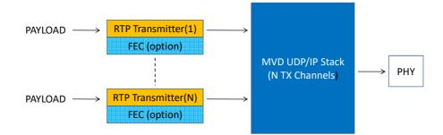
N parameter vary from FPGA ressources, Ethernet Speed connection and Number of Transmission channels requested.
