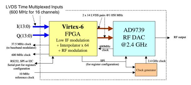
Much more and higher speed DSP functions can be implemented on the Virtex families. For example, with a single FPGA, a complete application for 32 to 64 DVB (or J83B) channels can be implemented from ASI or SPI input to RF output can be implemented.
