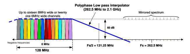
By taking advantage of the Spartan-6 unprecedented features on low cost FPGA architectures, this design fits into one of the smaller available part : XC6SLX16. For multi-channel application, this example however requires that the several I and Q channels are modulated at a low Intermediate Frequency, as shown in the figure. MVD Cores can provide technical assistance and/or complementary DSP functions for this.
