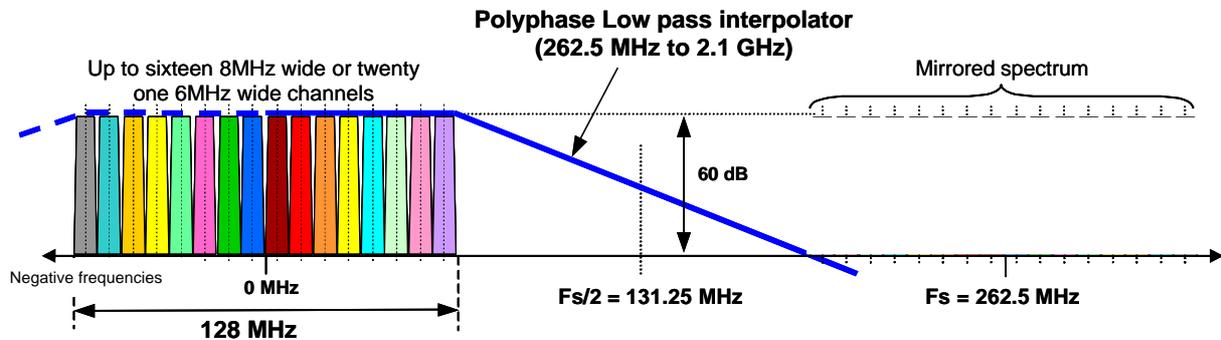
By taking advantage of the Spartan-6 unprecedented features on low cost FPGA architectures, this design fits into one of the smaller available part : XC6SLX16. For multi-channel application, this example however requires that the several I and Q channels are modulated at a low Intermediate Frequency, as shown in the figure. MVD Cores can provide technical assistance and/or complementary DSP functions for this.
